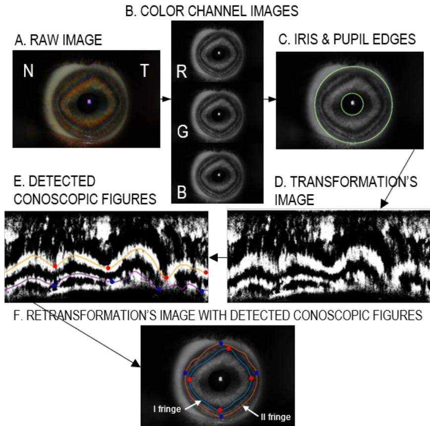
Figure 1. Block diagram of image analyzing process. Raw image (1A) is separated into color channel images (1B), the iris and pupil borders are distinguished (1C), the image is transformed into a polar system (1D), the lines responsible for isochromatics are detected as well as the inflection points (red and blue dots) (1E) after which lengths of the sides and angles are detected (1F)
